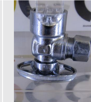
Figure 15. Angle stop valve, Day 200 Fresh water.
