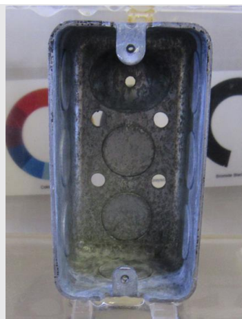
Figure 24. Junction Box, Day 200, Fresh Water
