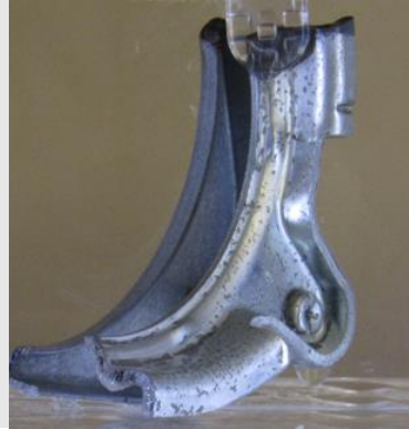
Figure 2. Garbage Disposal Bracket, Day 13, Fresh Water
