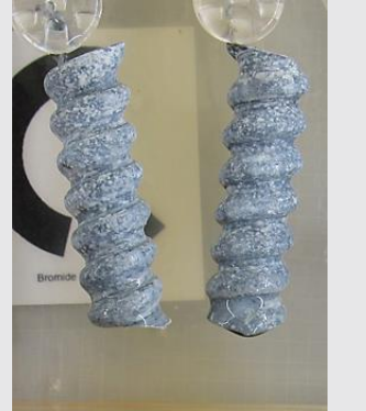
Figure 22. Flexible Electrical Conduit, Day 560, Saltwater.
