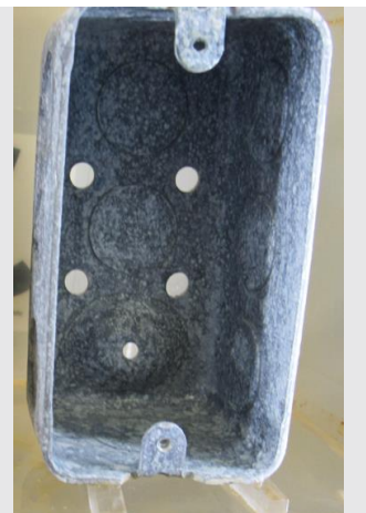
Figure 25. Junction Box, Day 560, Salt Water.
