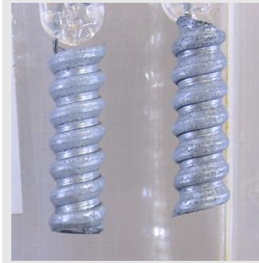
Figure 20. Flexible Electrical Conduit, Day 14, Freshwater.
