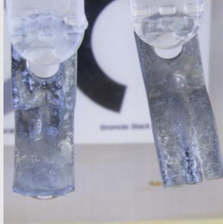
Figure 12. Electrical Conduit Strap, Day 200 Fresh Water.
