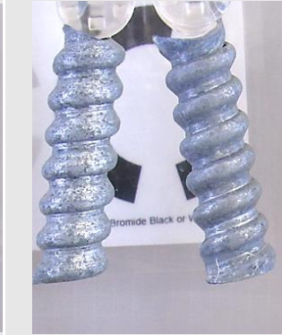
Figure 21. Flexible Electrical Conduit, Day 200 Freshwater.
