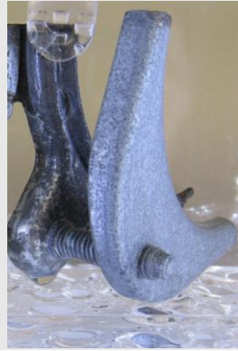
Figure 3. Garbage Disposal Bracket, Day 200, Fresh Water
