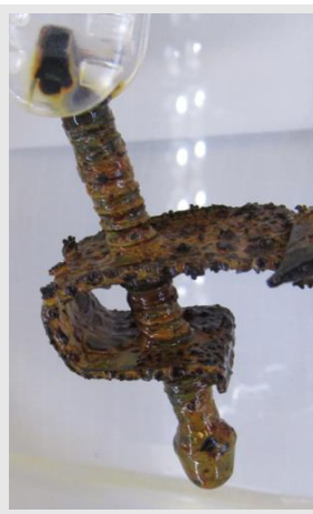
Figure 9. Steel Sink Fastener, Day 200, Fresh Water.
