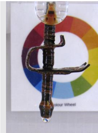
Figure 8. Steel Sink Fastener, Day 14, Fresh Water.
